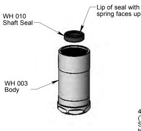
4. If you have a Fill Tube (TJ 064), insert it thru the Shaft Seal in the Body up to it's shoulder. Pour Viscous Fluid into the Body about 1" deep. Insert the Shaft into the you do not have the Fill Tube, insert the Shaft into fluid into the Body; allow the fluid to settle down thru the top bearing and about 10 minutes to get the tool full.
